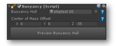
The Buoyancy Hull is the mesh referenced by the water simulation to determine how much of the mesh is submerged and how forces should be applied. This should be similar to a mesh collider, **but it should be as cheap as possible**. Buoyancy simulations are expensive - reducing the number of triangles that need to be accounted for goes a long way. To see your Buoyancy Hull in the editor, just hit the "Preview Buoyancy Hull" button.
