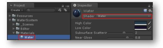
To apply the Water Shader, just drag it on top of your water plane in the scene view, or assign it in the Mesh Renderer component.
